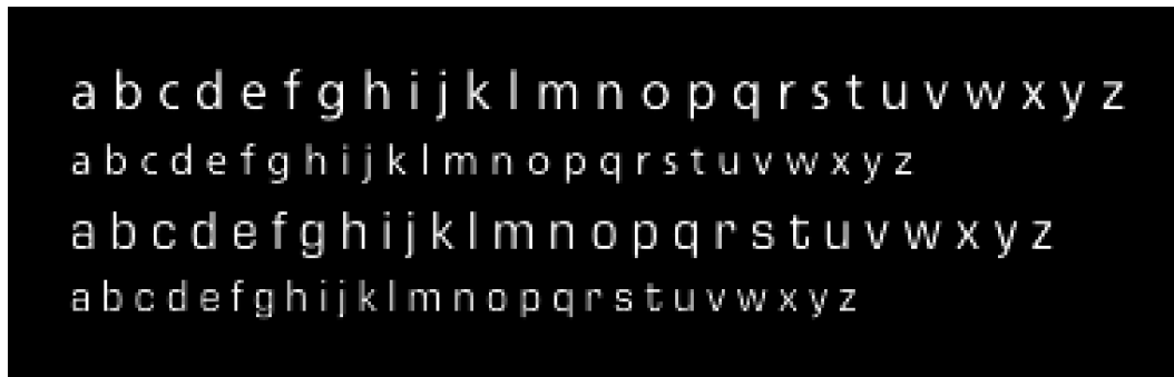
Figure 4: Samples of typefaces as displayed in actual screen pixels at 4mm (13 pixel capital height) and 3mm sizes (10 pixel capital height) for humanist (top 2 rows) and square grotesque (bottom 2 rows). Image taken directly from the Psychtoolbox frame buffer, zoomed to show rendering artifacts.
